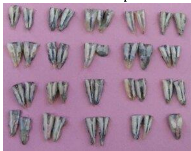
Figure 3. Glass ionomer samples prepared to study of linear color penetration rate by a stereomicroscope
